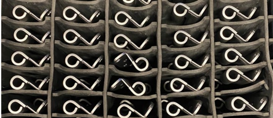
Parts in wrong orientation
